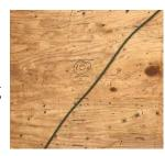
Photo showing dimensions of decking nail used (min. diameter 0.113 in. and min. length 2 3/8 in)
